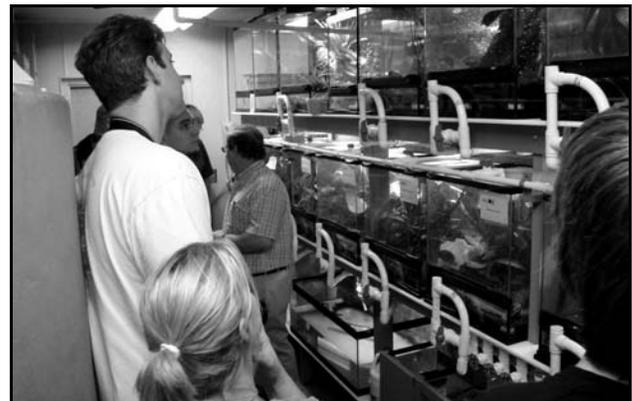
The staff designed and built an inexpensive system of PVC standpipes and valves to make it easy to regulate water levels in the amphibian tanks. Photograph by Dick Buchholz.
